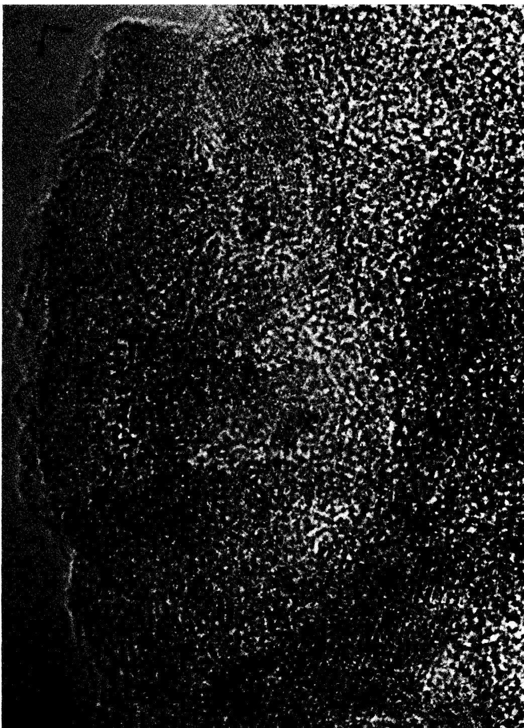
FIG. 5. Region of Catalyst B showing lattice fringes in several Pt particles (examples at X and Y) as well as the \gamma - \text{Al}_2\text{O}_3 support. A small region of (100) projection of \gamma - \text{Al}_2\text{O}_3 is indicated.
