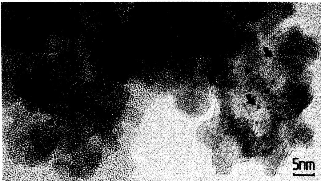
FIG. 1. Region of the "fresh" platinum/alumina catalyst after initial reduction in flowing hydrogen at 400^\circ C for 3 hr. The size of the Pt particles (some are arrowed) is indicated by comparison with the 0.46-nm (111) lattice fringes of \gamma-Al_2O_3 .
